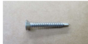
Fixed Panel Bracket Screw Fixed Panel to Jamb Screw #8 x 1 1/4" Flat Head Self Tapping
